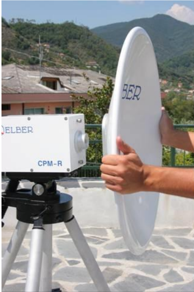
Figure 5: Parabolic dish fixing
