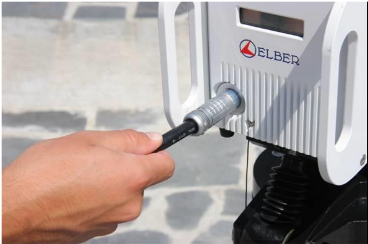
Figure 9: Connection of the RF head
