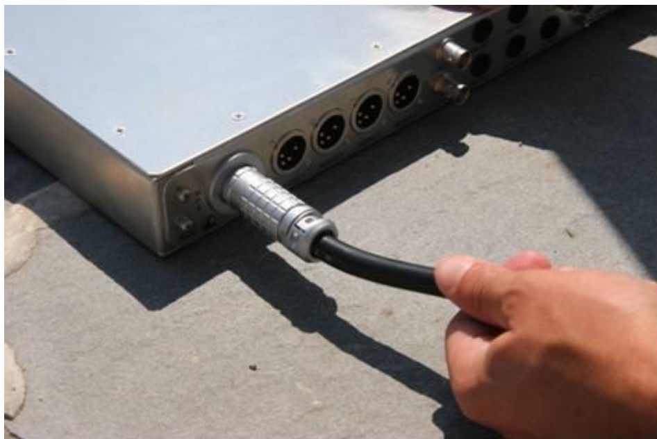
Figure 8: Connection of the control unit
